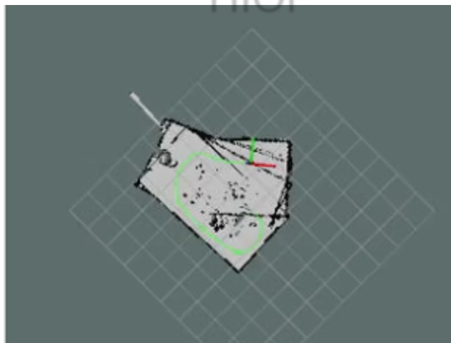
Figure 6.7: Not accurate when mapping in higher speed
