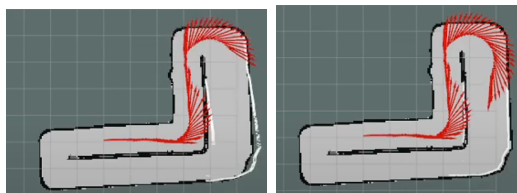
Figure 6.10: Trying to find position (white line out of place) and found position
